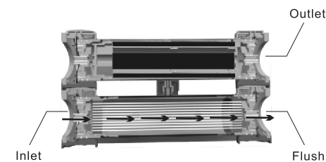
Pic.3 The principle of UF membrane flushing
